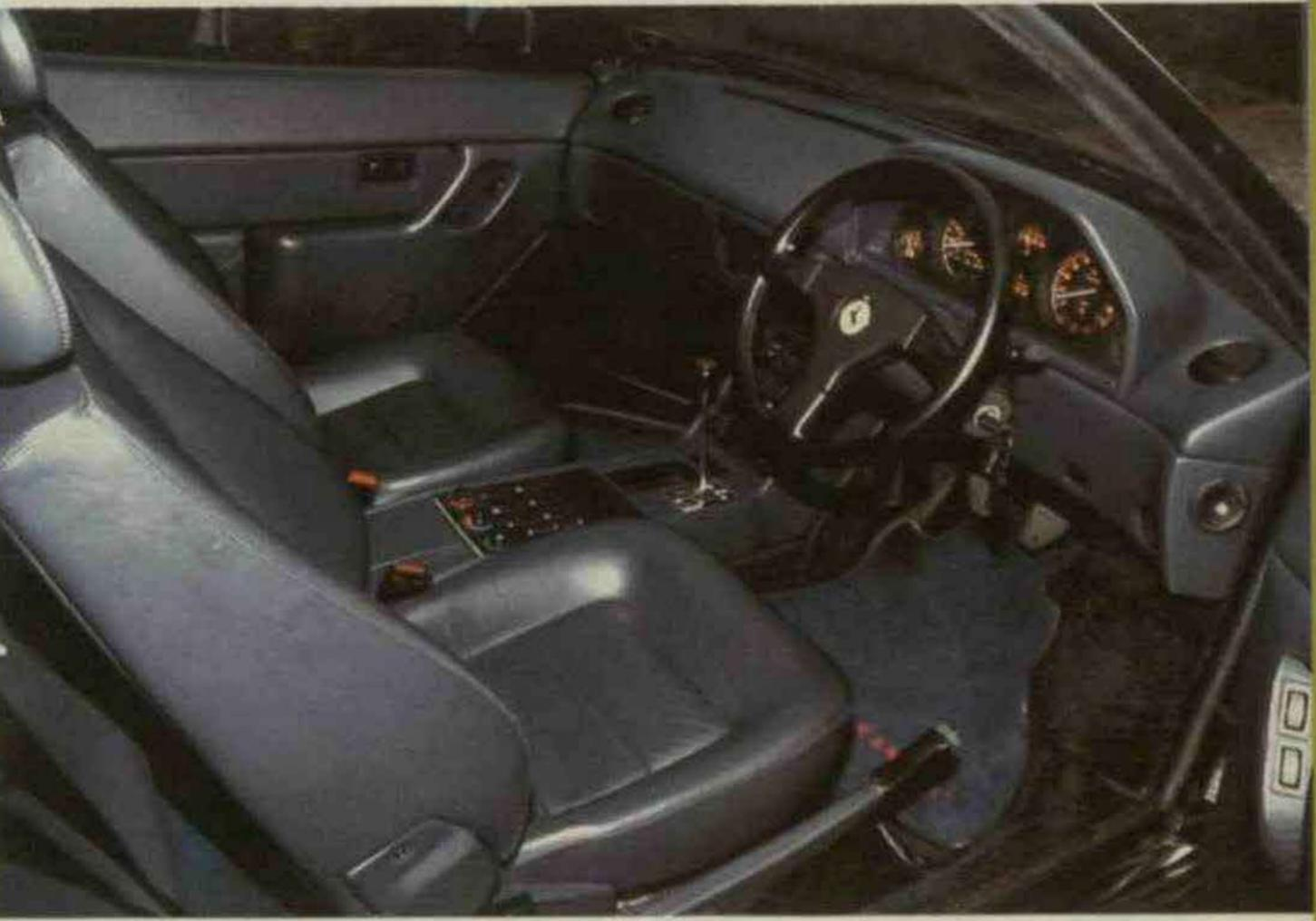
There was one overwhelming cold start bugbear: the traditional Ferrari aversion to selecting second gear with anything other than steamy Agip temperatures. It sounds simple enough, just miss out second and take advantage of the excellent torque curve and closely stacked initial ratios (fourth and fifth are widely spaced) to putter along for the couple of miles that it takes to warm-up
