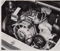
Capable of pushing the 911 to 60 mph in 6.61 sec, Porsche's air-cooled six has become a refined and smooth powerplant.
