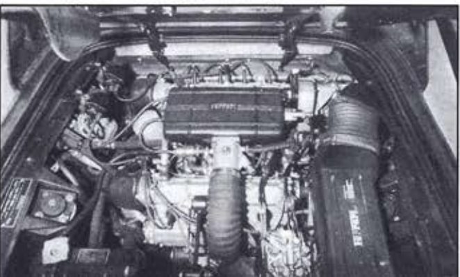
The 2926cc all-alloy four-cam V8 is derived directly from the GT4's but now has dual contactless ignition and Bosch K-Jetronic fuel injection
