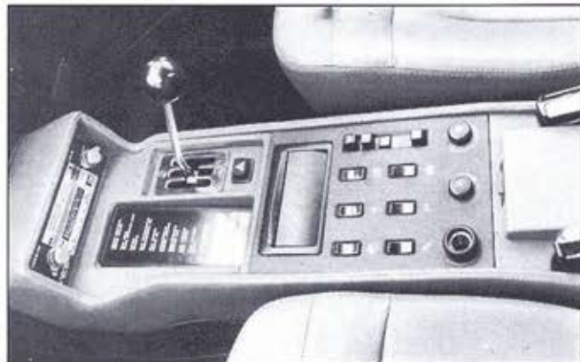
Above: redesigned central console houses the stereo, electronic check panel, and air conditioning controls, and electric controls for windows, glove box, aerial fuel filler. Rear seats, right, are comfortable but short on legroom
