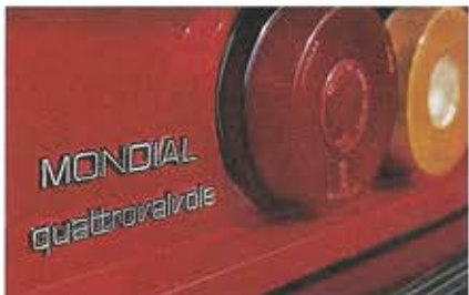
QV indicates 32 valve V8 and 28bhp extra
