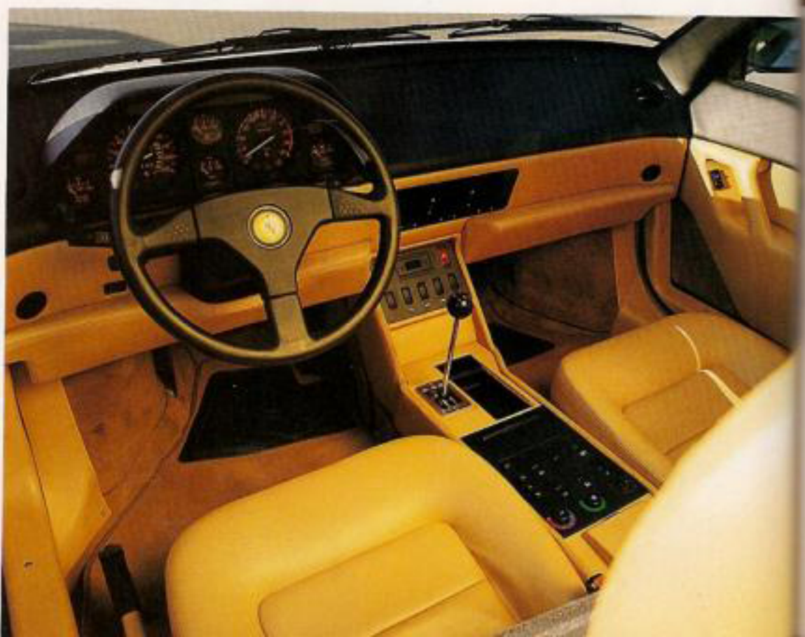
■ Ferrari interior is familiar, but clutch pedal is missing with Valeo automatic unit. Trunk holds tool kit.
