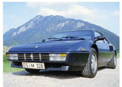
Integrated lamps on later, colour-coded nose (as this 3.2)
